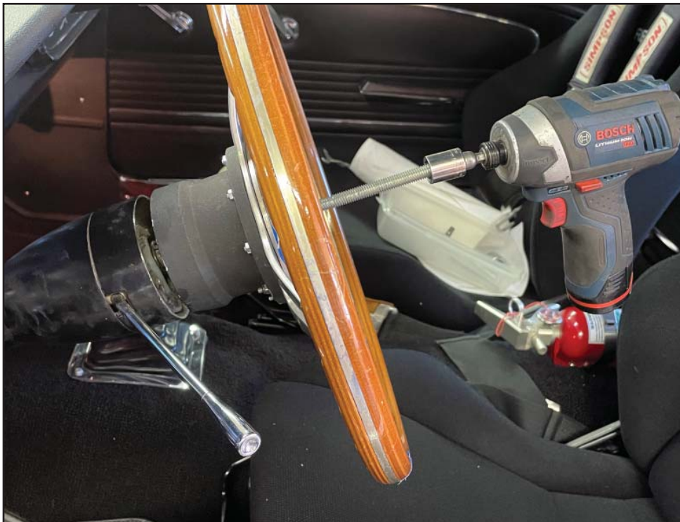
Once the end of the bolt touched the end of the shaft, a quick rattle was all it took to pop the hub and wheel free from the shaft
