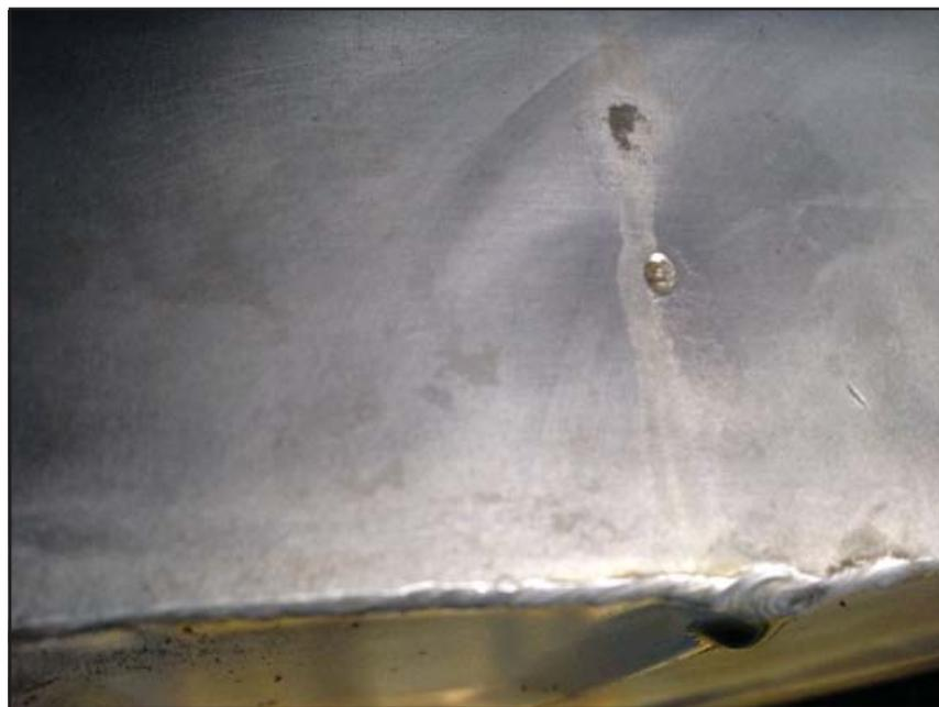
*After a good wipe-down, it was possible to see two spots where the internal weld had penetrated to the exterior of the pan. The top one had a pinhole, which is impossible to see with the naked eye*
