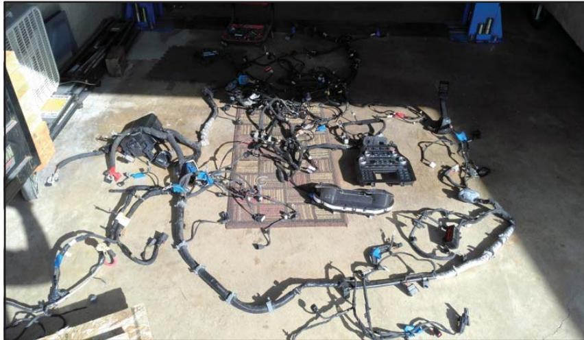
*The wiring harness has over 2500 individual connections!*
