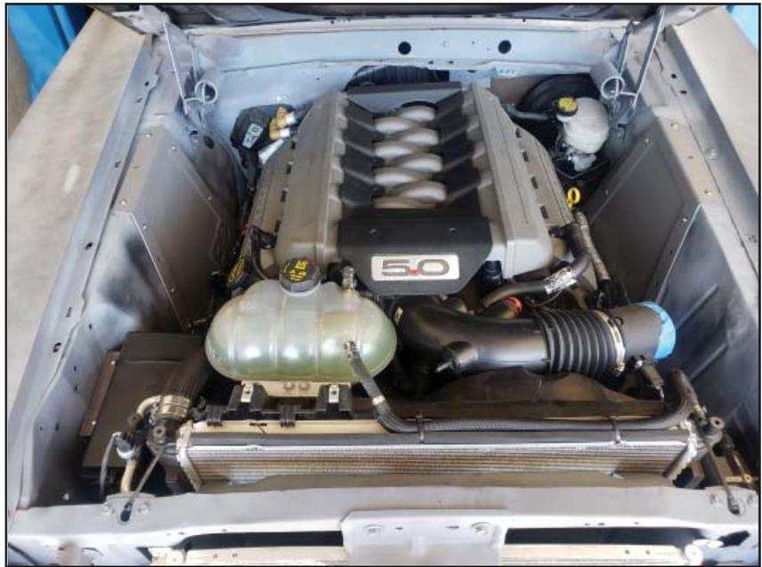
*The 5.0L (302 cubic inch) 'Coyote' V8 is based on the architecture of the 4.6L and 5.4L modular engines. It features a reinforced block, lowered intake plenum, and new 4-valve DOHC heads that shift the cams outboard and used roller fingers, which allows improved (raised) intake port geometry. It features twin independent variable cams, where the intake and exhaust cam timing can be advanced and retarded independently by the engine control module*
