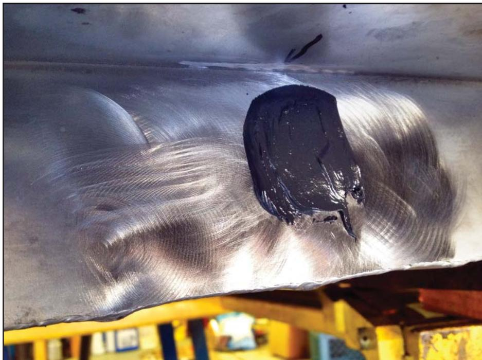
*The first coat of JB Weld certainly covered the known leak, but the spot just below it was slightly exposed, so after this photo was taken we elected to add a second, larger patch, just to be sure*
