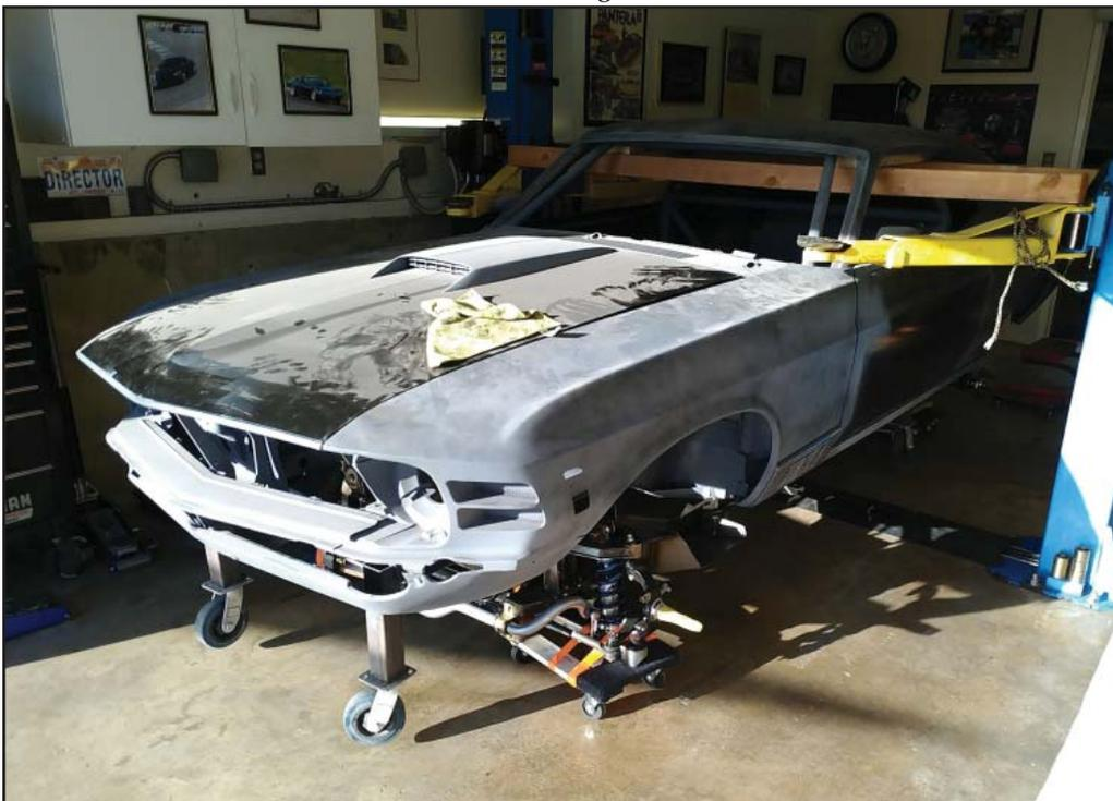
*I was able to hang the car by the roll cage, in order to assemble and install the suspension*
