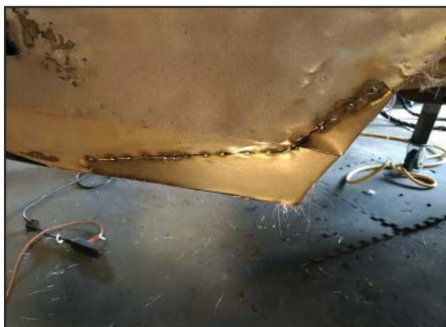
*After finding rust all over the car, hundreds of hours were spent cutting away bad metal and welding new metal in*
