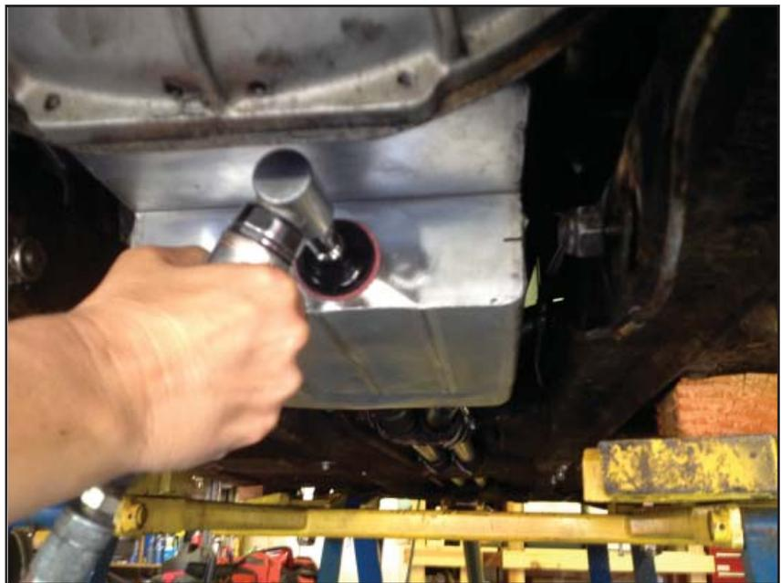
*After a thorough degreasing, Lori used an angle grinder fitted with a surfacing pad to scuff up the back of the pan to give the JB Weld a better surface to adhere to*
