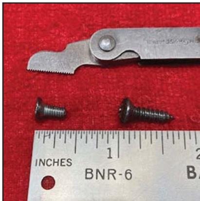
the plastic housings that surround the ignition switch and steering column? Oddly, these screws are completely different in type and character from one side to the other, and as there is lots of 12V running around in there, the potential pitfalls of using the incorrect/too-long screw are great.
