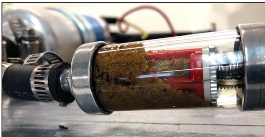
***The fuel filter was completely clogged after only three minutes! It required multiple iterations of sweeping and filter cleaning before he was done***
