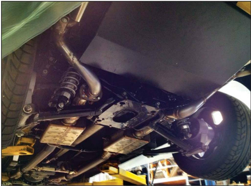
*Custom-fabricated oval exhaust system, stainless steel mufflers, fuel cell, Tremec gearbox, and De Tomaso Deauville independent rear suspension—this is no ordinary Shelby GT350 clone!*
