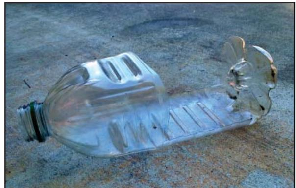
*Simply cut away three sides of a plastic jug to make a no-cost Pantera oil drain funnel*
