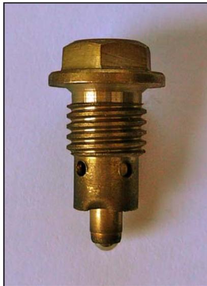
***The little ball at the bottom of this new needle valve assembly was not where it should have been in the old one***
