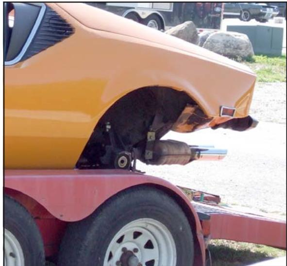
*This photo graphically illustrates what happens when axle wear goes undetected and unresolved. Close examination of the photo reveals the wheel bearing, plainly visible, with the snapped-off axle stub still inside.*
