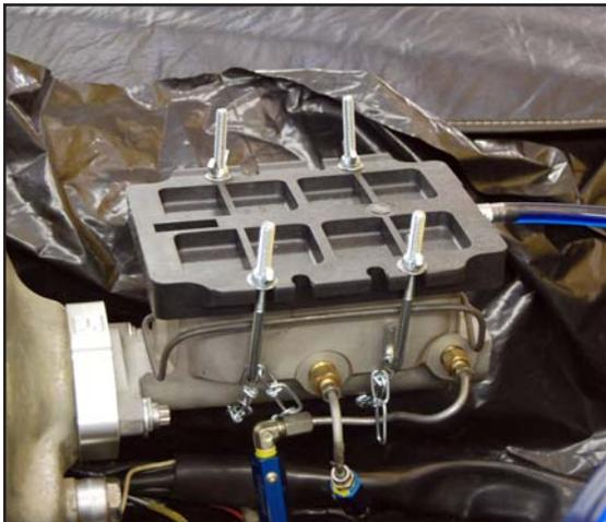
*The interface with the top of a standard Ford-style master cylinder is a bit hokey. The molded plastic plate has a soft rubber insert which seals against the top of the master cylinder; it's held in place using J-hooks and hardware store chain (all included with the adapter). A better solution is to place a block of wood at the adapter and compress it against the master cylinder with a large C-clamp*
