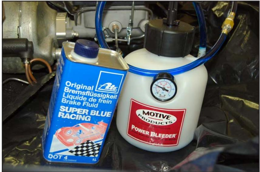
*The power bleeder is a small, simple unit consisting of a fluid canister with pressure gauge, hand pump, and a hose. ATE Super Blue Racing brake fluid is about the best you can get (for a reasonable price), and has the advantage of being bright blue in color*
