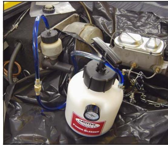
*The included adapter threads right onto the stock clutch master cylinder. Note the air pressure is a very reasonable 10 psi; you don't want any more than this, to minimize the threat of spraying fluid*
