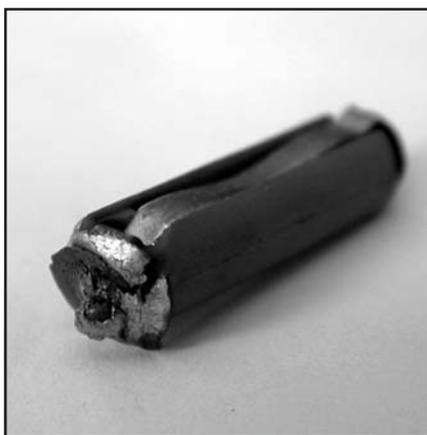
*This fuse appeared fine when it was in the fuse box, but closer inspection revealed that both ends were seriously melted and it was barely making contact*
