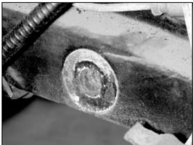
*The GT5-S frame rail is an incredibly simple piece, formed from a single piece of 14-gauge metal bent in a U-shape. The area where the lower control arm yoke mounting bolt penetrates receives zero external reinforcement—the circular pattern is abrasion from the fender washer*
