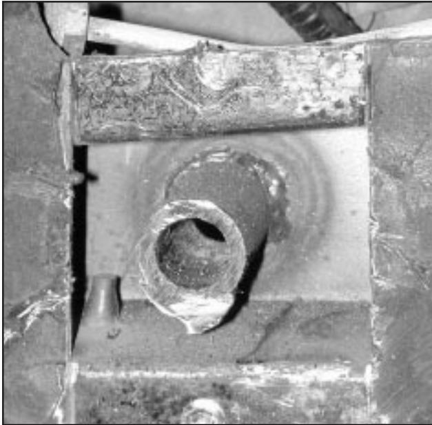
*Cutting open the side of a GT5-S frame rail from the outside (wheelwell) reveals a simple tube, welded around its entire circumference to the inner side of the inside portion of the frame rail. This tube was then affixed to the outer frame rail panel with one small mig weld at the bottom. The inner structure is none too strong; as you see this, one can grasp the end of this sort section of tube and wiggle it around as the inner frame rail sheet metal bends with strong hand effort.*
