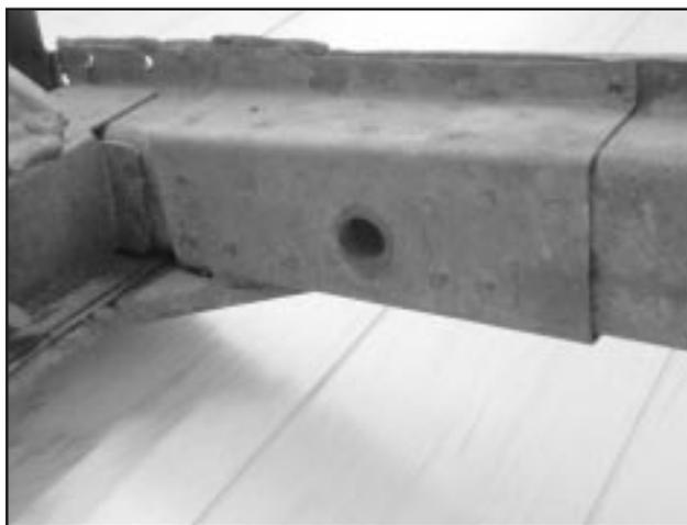
*In stark contrast, the Ford-era chassis benefits from extensive reinforcement in this area. A second piece of sheet metal is bent into shape, and encompasses the entire structure. It is spot-welded to the top and bottom flanges, and also receives numerous spot-welds to the underlying piece*
